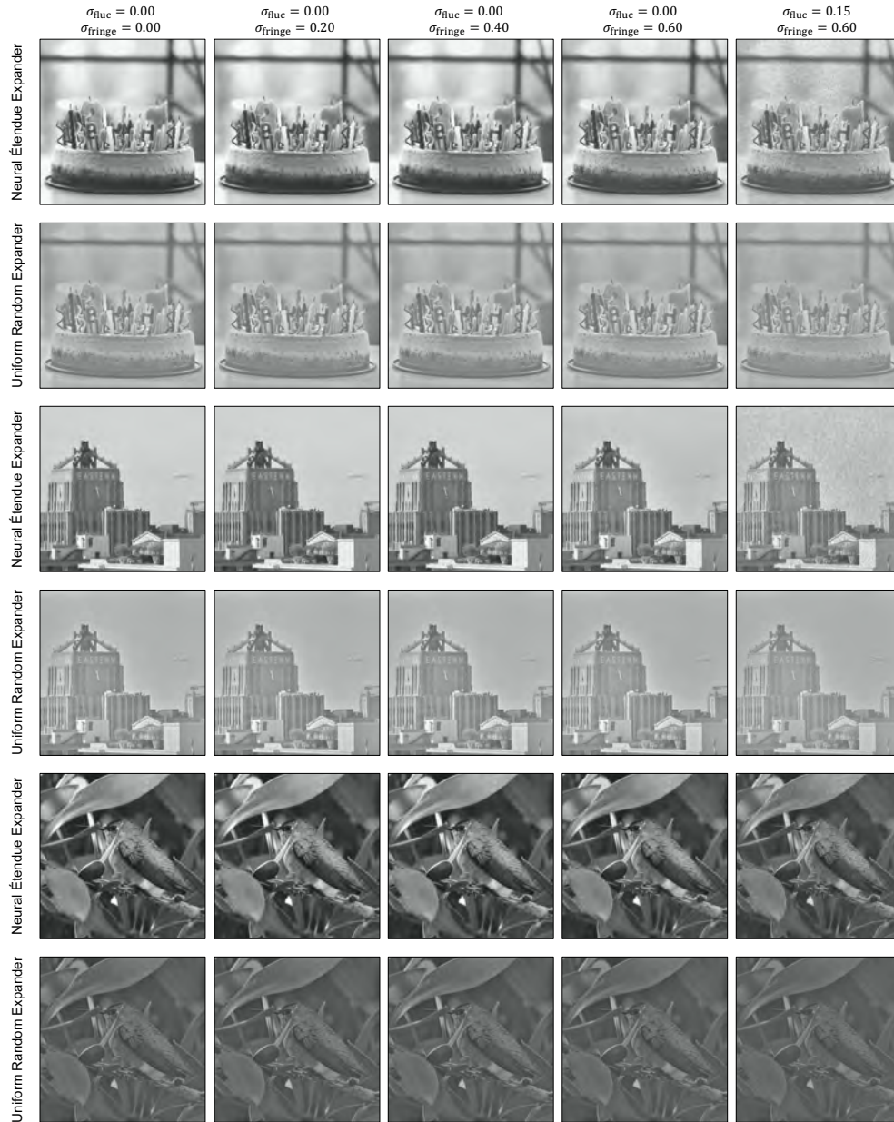
Figure S19: Impact of SLM non-idealities on hologram reconstruction. These holograms are simulated with increasing phase fringing error. The blur kernel used for simulating the phase fringing effect is a Gaussian kernel with standard deviation denoted by \sigma_{\text{fringe}} . The rightmost column shows the combined effect of phase fluctuation and phase fringing error. These holograms are simulated at 64\times étendue expansion.
