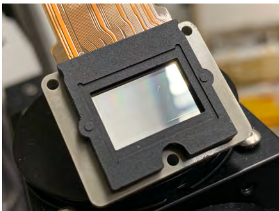
Figure S24: Photographs of the fabricated DOEs. This picture shows the stamped resin on top of the glass substrate. A picture of the SLM is shown for comparison.
