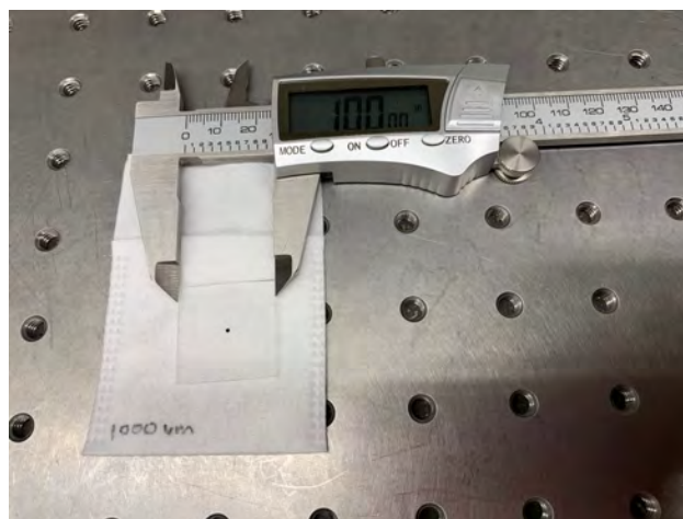
Figure S27: Picture of a DC block. We fill the center of a square piece of glass with a chrome filling. The chrome blocks out the undiffracted DC component of the SLM when placed at the Fourier plane of the 4F system. The diameter of the chrome filling shown in this picture is 1000 \mu\text{m} . For the hardware prototype we used a DC block which has a chrome filling with a smaller diameter of 100 \mu\text{m} .
