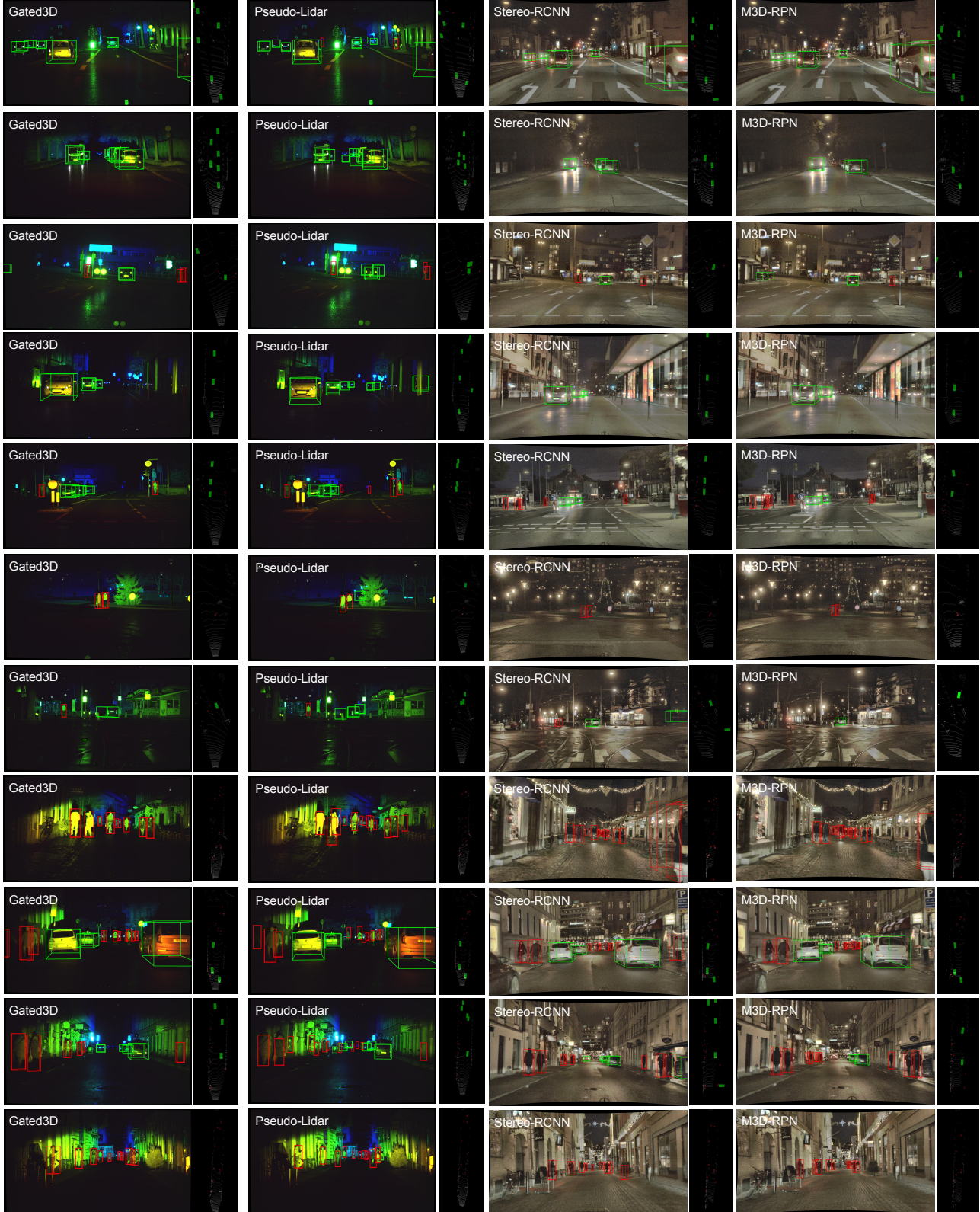
Figure 1: Qualitative comparison against baseline methods on the captured dataset. Bounding boxes from the proposed method are tighter and more accurate than the state-of-the-art methods. The BEV lidar overlays show that our method offers more accurate depth and orientation than the baselines. The advantages of our method are most noticeable for pedestrians, as cars are easier to detect for other methods due to being large and specular (please zoom in on the electronic version for details).
