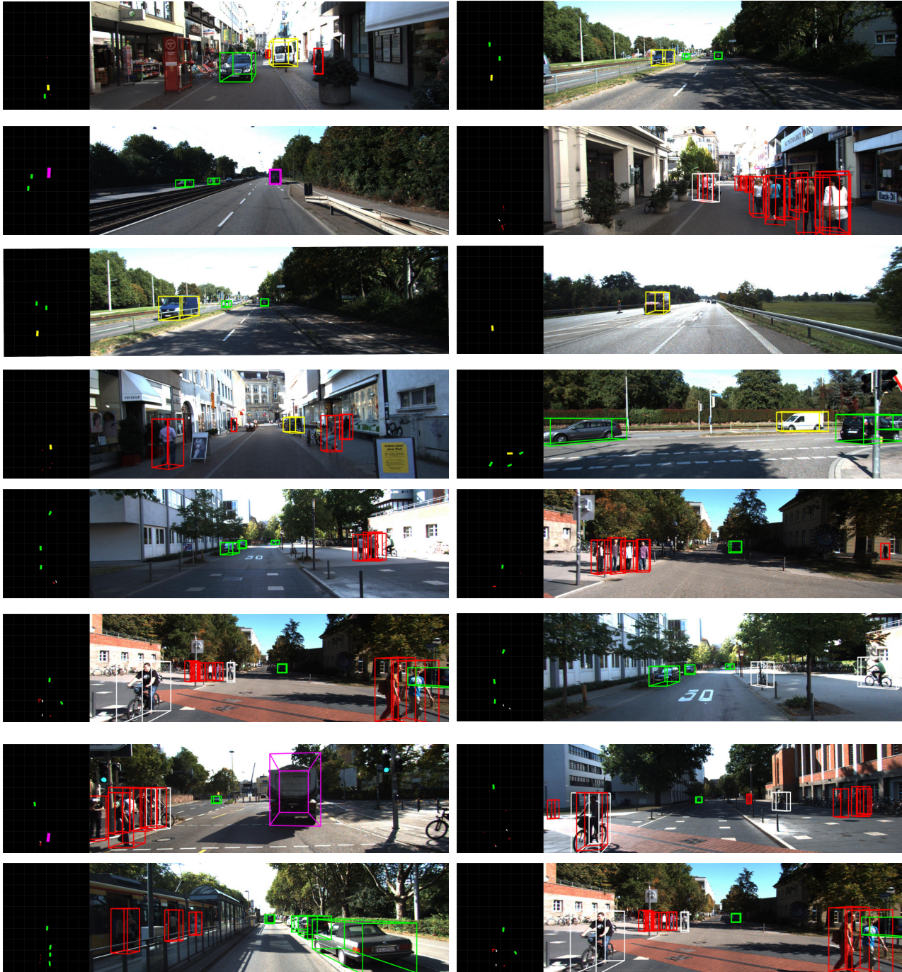
Figure 2: Generalization Experiment: Although our model has not been optimized for RGB data, it generalizes to KITTI RGB data, see text. We present qualitative results of our Gated3D model applied to RGB from KITTI validation (top four rows) and test (bottom four rows) sets. 3D boxes are color-coded as green=Car, yellow=Van, purple=Truck, red=Pedestrian, white=Cyclist. BEV shows an area in the [0m, 100m] and [-40, +40m] ranges in the Z and X camera coordinates, respectively. Our model effectively recognizes objects of varying dimensions and types, i.e. Cars, Vans, and Trucks.
