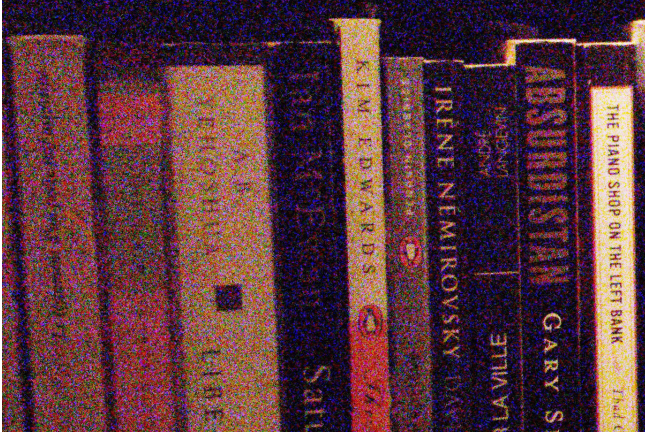
Fig. 2. A RAW frame captured indoors using a Nexus 6 rear camera (after demosaicking). The image was taken at ISO 3000 with a 32 ms exposure time. The noise in the image is clearly visible.
