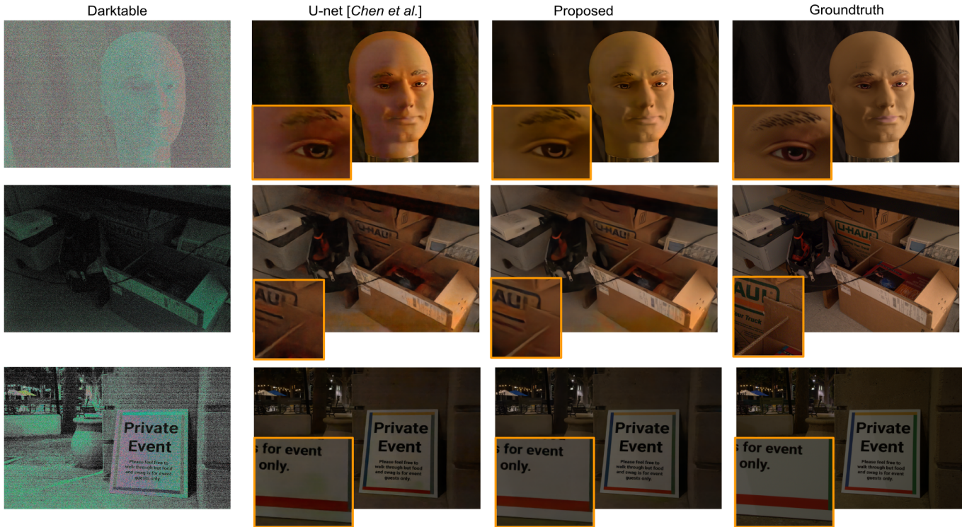
Fig. 6. Anscombe Networks for Single-Image Low-Light Photography (w/o Classification). Qualitative low-light denoising results for human viewing using the traditional Darktable ISP, the U-Net model proposed by [Chen et al. 2018], and the proposed Anscombe network. The proposed model and Chen et al. [2018] have been trained on the same low-light dataset from the dataset proposed in [Chen et al. 2018]. All methods use the same single RAW image as input.
