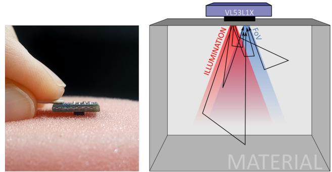
Fig. 4. For the material measurement, the VL53L1X is placed in direct contact of the sample. The active illumination penetrates the material and is scattered inside as illustrated on the right. Depending on the material’s structure, the signal measured by the SPAD sensor varies spatially and temporally.
