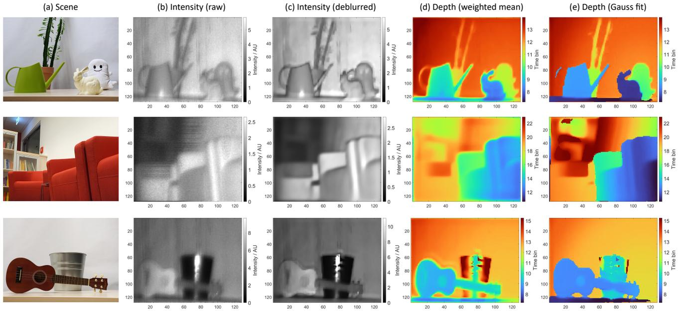
Fig. 12. Measurements taken with our scanning setup of three different real scenes shown in column (a). Column (b) shows the measured intensity of each pixel as raw data. After applying several corrections to the data, we obtain clearer and less noisy data as shown in (c). From this data, depth maps are calculated in two different ways, once as a weighted mean as shown in column (d), and once by fitting Gaussian distributions to the measured histograms (column (e)).
