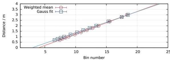
Fig. 13. Calibration of the relation between bin number and true distance for both methods used to determine the position of the depth peak.
