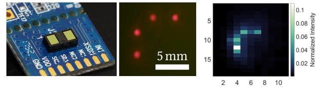
Fig. 3. Left: The VL53L1X time-of-flight sensor module by STMicroelectronics on a commercially available breakout board. Center: Profile of collimated laser beam at 0.4 m from the lens. Right: Point spread function of the full system shown in Figure 2, obtained using a small retroreflective target.
