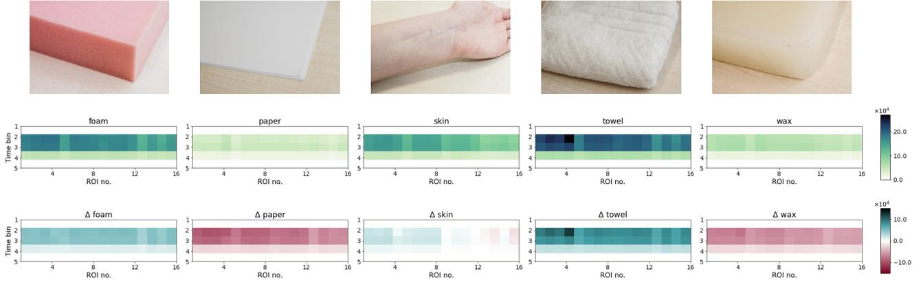
Fig. 5. Measurements for five different materials. Top: Photograph of material. Center: SPAD histogram data averaged over 1000 measurements. Bottom: Deviation of each material from the mean of all materials. *Center and bottom: Since no visible information is contained in later time bins, these plots only show bins 1 to 5.*
