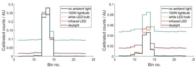
Fig. 14. Exemplary histograms for a bright (left) and a dark (right) scene pixel (after intensity calibration using the first five bins of the raw histogram) for different ambient light scenarios (no ambient light, a 100 W incandescent lightbulb, a 230 lm white LED lightbulb, a 940 nm infrared LED, and indirect daylight through an open window).
