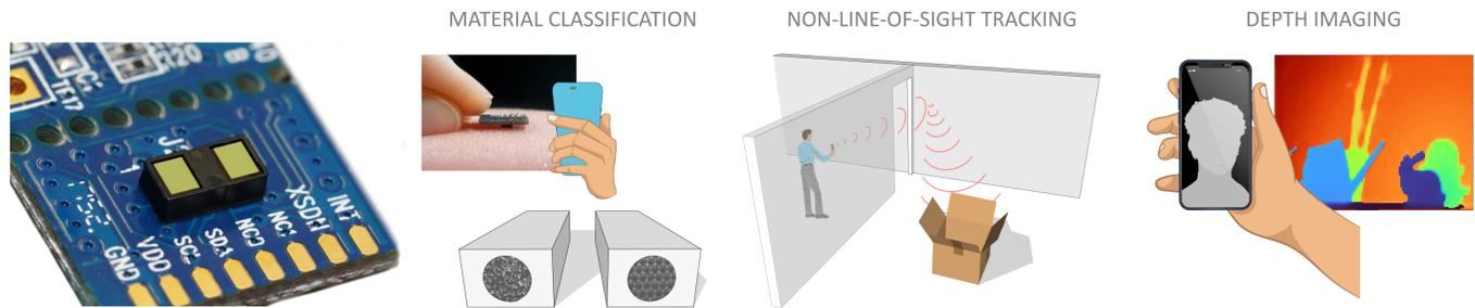
Fig. 1. We propose the use of cheap, small off-the-shelf distance sensors (far left) for a variety of computational imaging and vision tasks, and demonstrate and evaluate their capabilities in emerging sensing applications like (from left to right) material classification, non-line-of-sight tracking, and depth imaging.
