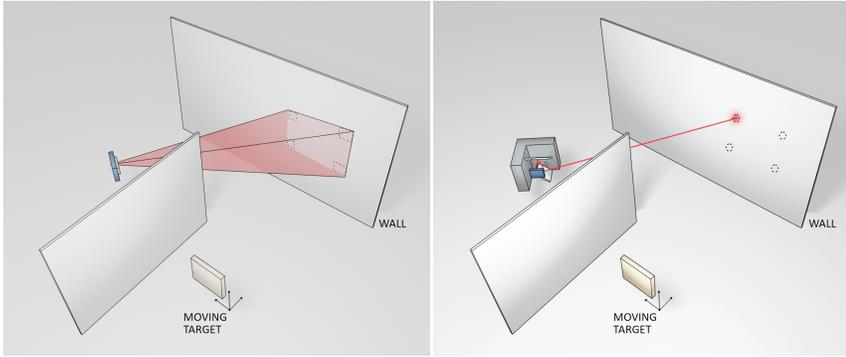
Fig. 8. Two variants of NLOS tracking setting. Left: The SPAD package’s integrated light source directly illuminates the wall in front of the occluded target. The histograms from the four corners of the SPAD image are read out. Right: The illumination and SPAD view is collimated using the *glasses* and deflected to four points on the wall using a mirror galvanometer.
