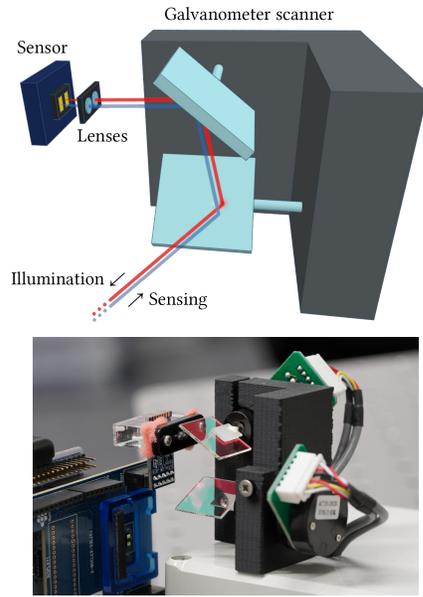
Fig. 2. Top: Setup schematic for depth and NLOS imaging: Two plano-convex lenses collimate the light emitted from the VL53L1X’s light source and the SPAD sensor’s field of view. Two rotatable mirrors allow deflection of the beam. Bottom: Lenses and galvanometer scanner pair in front of the sensor and light source in the lab.
