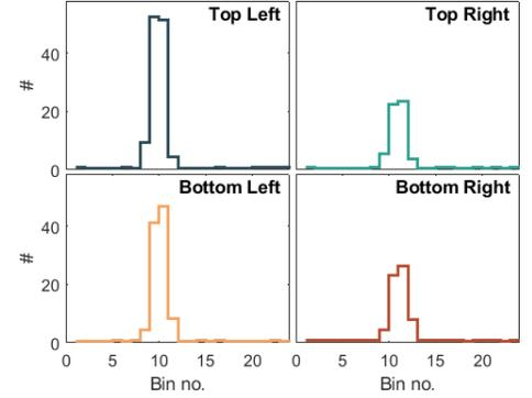
Fig. 9. Histograms for all four corners measured with the setting without mirrors for one target position, averaged over 30 measurements. The peaks from the reflection on the wall are clearly visible.
