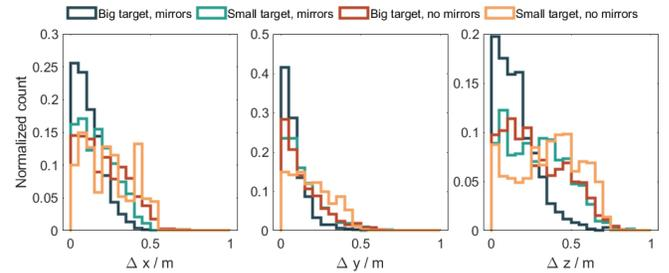
Fig. 10. Distances in all spatial dimensions between the true and predicted target position in the test dataset for the ‘direct position prediction’ method.
