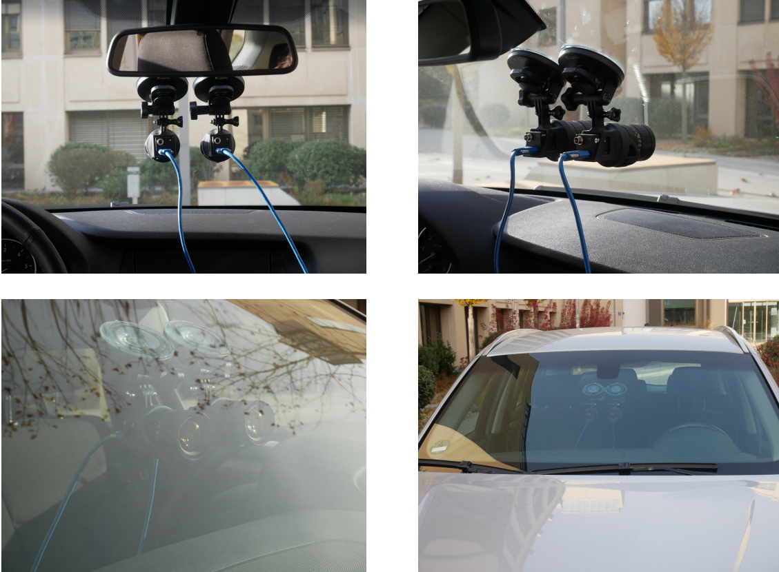
Figure 1: Vehicle Prototype. We mount two cameras with free-running auto-exposure side-by-side on the windshield of a testing vehicle. The detections of the two separate camera systems are independently annotated for a fair comparison and evaluation.
