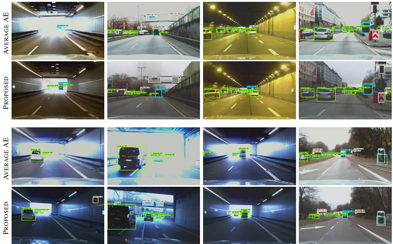
Figure 2: Experimental prototype results of the proposed neural AE compared to the Average AE baseline method using the real-time side-by-side prototype vehicle capture system shown in Fig. 1. The proposed method accurately balances exposure between objects and adapts itself robustly to changing conditions.
