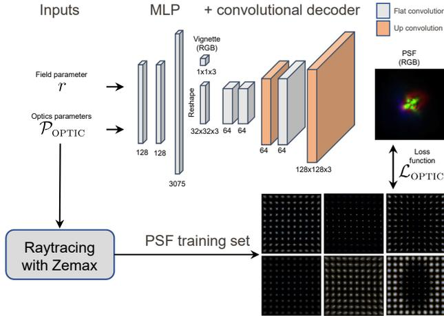
Fig. 5. Overview of our optics meta-network training procedure. We train our optics meta-network to map  $\mathcal{P}_{\text{OPTIC}}$  and  $r$  to spatial PSFs. We use spatial PSF training data acquired by driving ZEMAX’s ray tracer with  $\mathcal{P}_{\text{OPTIC}}$ .
