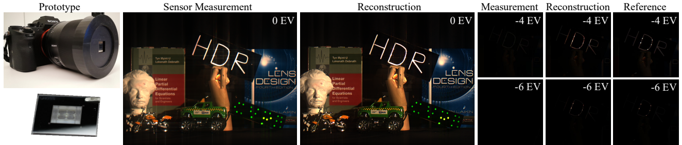
Figure 1: Due to pixel saturation, image detail in bright regions is lost in a single snapshot LDR image. Our camera, with the learned optic prototype (left), captures LDR images where high-intensity image content is encoded through a series of streaks (center left). This allows us to reconstruct the lost highlights (center, center right) with a specialized two-stage CNN.
