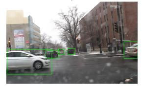
Figure 6: ARM MALI-C71 ISP for 2D automotive object detection example in snowfall condition.
