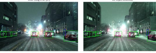
Figure 8: ARM MALI-C71 ISP for 2D automotive object detection example in night snowfall conditions.
