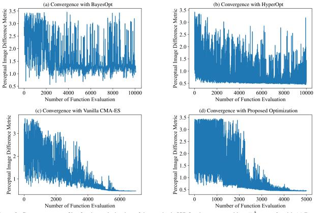
Figure 3: Convergence profiles for the optimization of the synthetic ISP for the perceptual loss  $5\hat{\mathcal{L}}_{PERC} + \ell_1$  with (a) BayesOpt [20], (b) HyperOpt [5], (c) Vanilla CMA-ES[16], and (d) the proposed optimization method.
