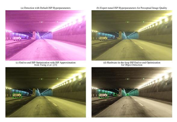
Figure 4: ARM MALI-C71 ISP automotive 2D object detection example in a tunnel. With the ISP optimized using the proposed hardware-in-the loop approach, noise is visible; however, the object detector manages to detect smaller objects with this ISP hyperparameter setting than with hyperparameters obtained with alternative methods, presumably because smoother images have less detail.
